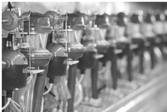
Inline devices for milk component analysis are a valuable tool for detecting ketosis and other metabolic conditions.
